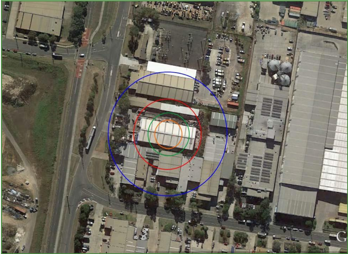
Figure 11.9. Heat Radiation Contours for Scenario B1: Fire involving 700 T of Cardboard. Note: Isopleths illustrate the heat of radiation contours: Blue = 4.7 kW/m 2 ; Red = 12.6 kW/m 2 ; Green = 23 kW/m 2 , Orange = 35 kW/m 2 .
