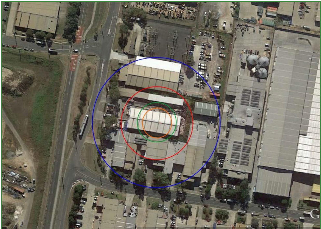
Figure 11.11. Heat Radiation Contours for Scenario C1: Fire involving 1000 T of Cardboard. Note: Isoleths illustrate the heat of radiation contours: Blue = 4.7 kW/m 2 ; Red = 12.6 kW/m 2 ; Green = 23 kW/m 2 , Orange = 35 kW/m 2 .
