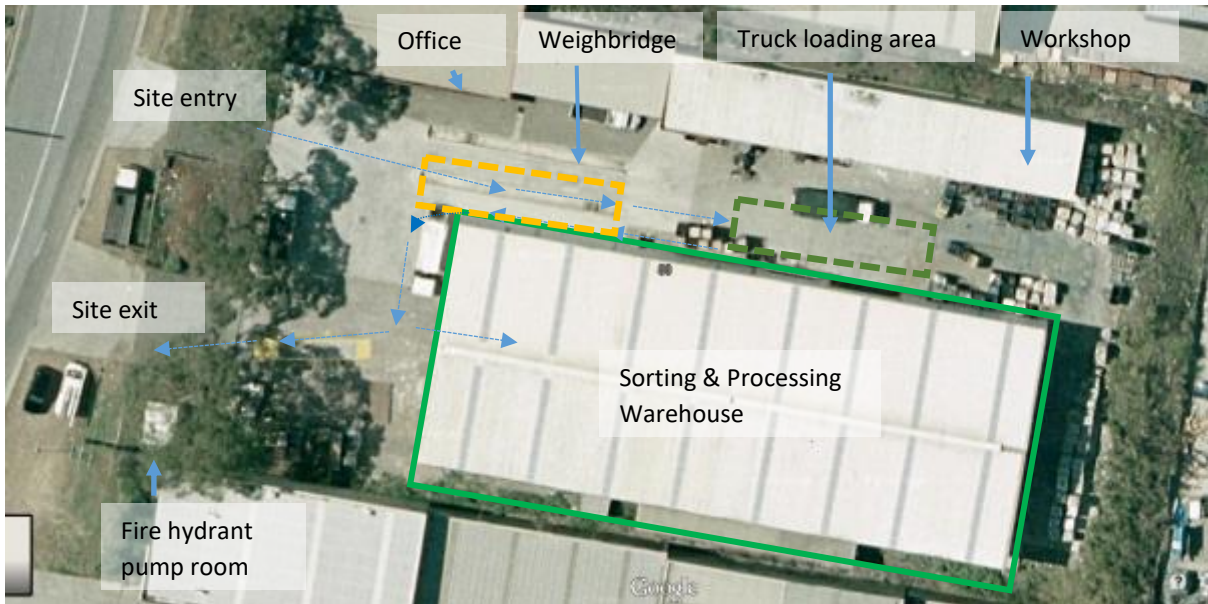
Figure 2.3. Detailed site layout of current operation, including vehicle movements.
