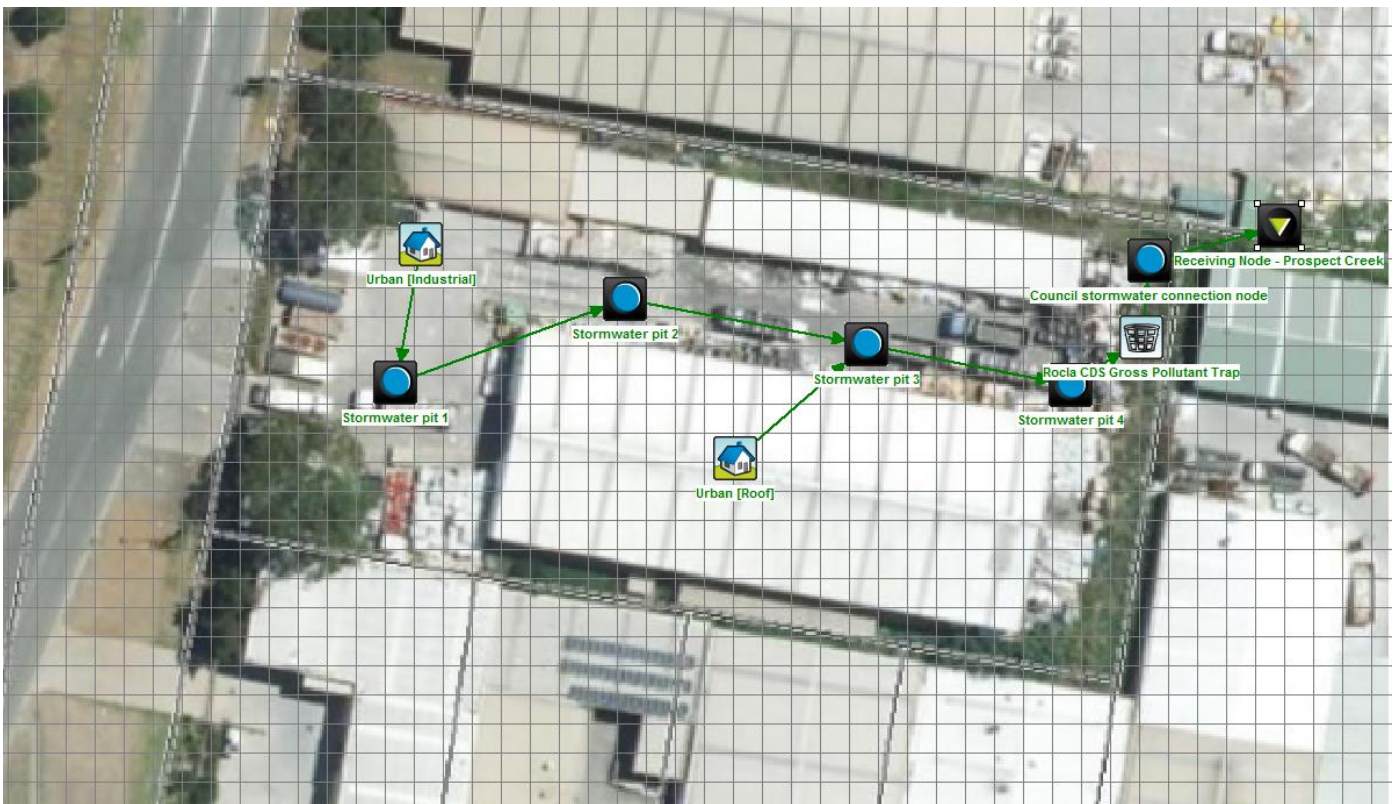
Figure 6.8. Post-development stormwater model and treatment train. Note that the receiving waterway is Prospect Creek (MUSIC v6.2.0).
