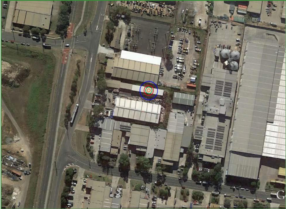
Figure 11.8. Heat Radiation Contours for Scenario A1: Fire involving 100 T of Plastic. Note: Isoleths illustrate the heat of radiation contours: Blue = 4.7 kW/m 2 ; Red = 12.6 kW/m 2 ; Green = 23 kW/m 2 , Orange = 35 kW/m 2 .
