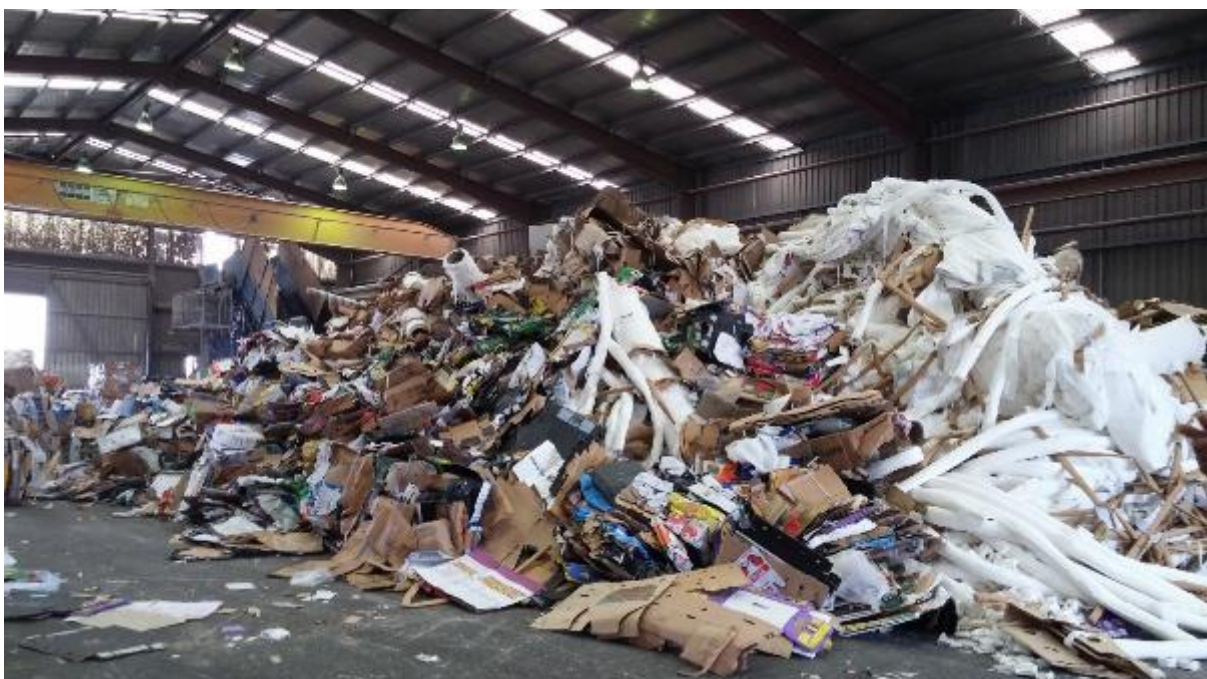
Figure 2.6. Unloading area of recovered paper, cardboard and plastic film in the warehouse. Trucks after being weighed on the weighbridge enter the warehouse where the materials are inspected and sorted where required.
