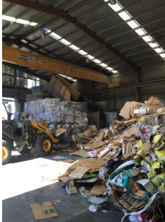
Figure 2.7. Baling of cardboard into blocks (top photo). Loading of blocks of baled cardboard onto waiting truck for transport to recycling markets (bottom photo).
